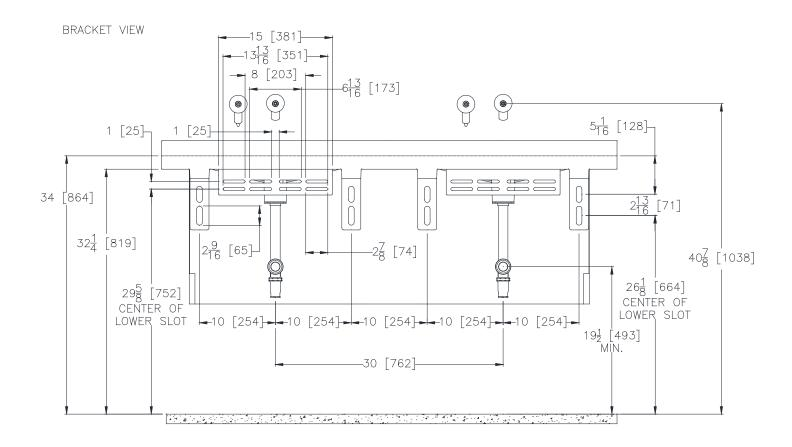
Installing the P-trap outlet lower than 19.5" from the finished floor will prevent the vandal shroud from being installed.
