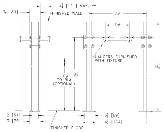
\*\* WITH STANDARD STUD LENGTH OF 6. # REFER TO ROUGH-IN GUIDE OF SPECIFIC FIXTURE FOR DIM.
