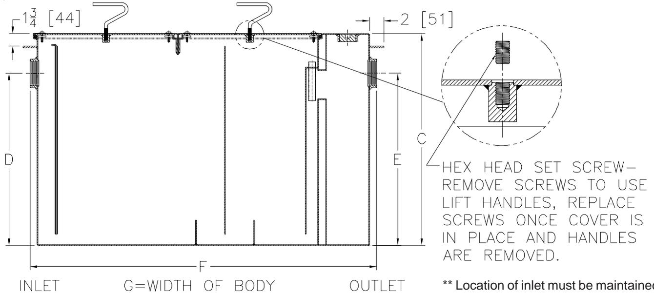
\*\* Location of inlet must be maintained at the 'D' dimension listed for each size.
