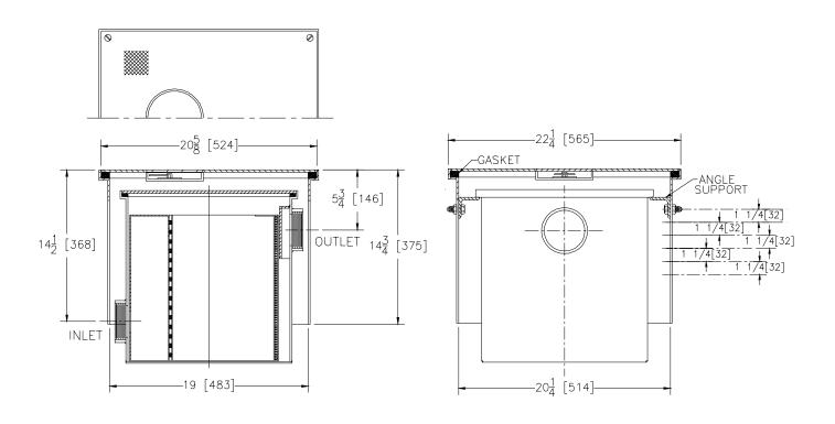
**ENGINEERING SPECIFICATION**: ZURN Z1181-R Acid Resistant Epoxy Coated Recessing receiver equipped with adjustable support brackets and gasketed non-skid cover with recessed and covered lift handle. Complete with Z1181 solids interceptor for solids interceptor specifications see Z 1181 drawing.
