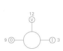
Inlet (I), Outlet (O) and Vent (V)
