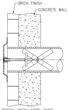
TYPICAL INSTALLATION USING PIPE CLAMP HARDWARE
