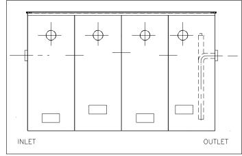
heavier materials are retained in the first compartment, while smaller and lighter materials are trapped in other compartments. Oil, grease, and similar materials will be retained at the surface of some or all eight compartments. Any gaseous fumes will be collected between the top of the water and the bottom of the cover and vented through the four individual 2" [51 mm] threaded vent connections.
