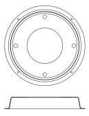
Z1035 (For 8-3/8" diameter drain body.)
