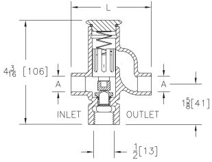
**Note:** Trap primer should be installed a minimum of 6" above grid of floor drain or flood level rim of equipment served.
