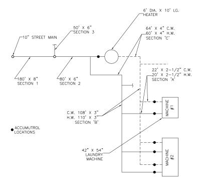
Piping Data (From Machine to Heater)
