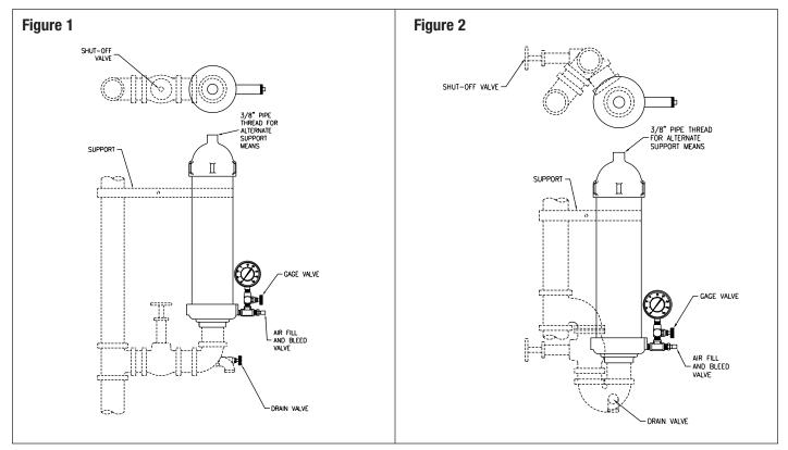
NOTE: Dotted lines indicate items by others. Accumutrol shown on vertical supply line. On horizontal supply, mount Accumutrol vertically and use same fitting and valve arrangement.
