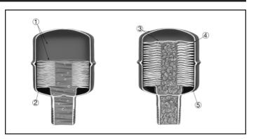
All-Stainless-Steel Construction – When sized properly, the Shoktrol's bellows cannot take a permanent set even if expanded by static line pressure for prolonged periods, nor split or tear under stress. Exterior requires no additional treatment to blend with surroundings on exposed installations.
