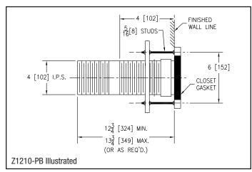
**-PC** Coupling Connection with 4" [102mm] Cleanout for Penal Fixtures (Z1214 and Z1215)
