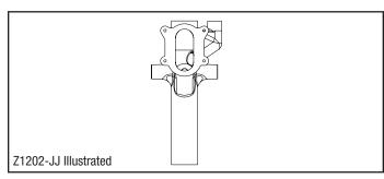
**-JL** 2" [51mm] Left-Hand Auxiliary Inlet (Z1202-N4, Z1202-ND4, Z1202-H4, Z1202-HD4, and Z1202-1HR4)
