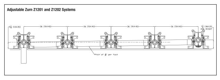
For installation of fixtures, up to a ten fixture maximum, either side of stack fitting:
