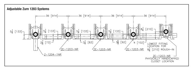
For installation of fixtures, up to a ten fixture maximum, either side of stack fitting:
