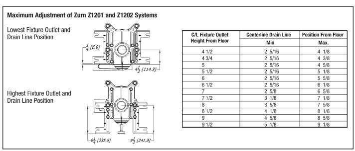
For any given rough-in height, the fitting can be adjusted up and down (a maximum of 4" [102mm]) to accommodate drainage pitch on long runs. When back-to-back and handicapped rough-ins are used, note that there are further limitations to the number of fittings in a given run.
