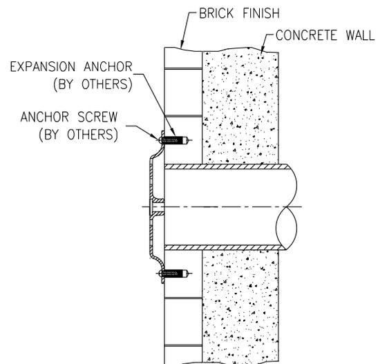
TYPICAL INSTALLATION USING FLANGE MOUNTING HOLES (-LC SUFFIX)
