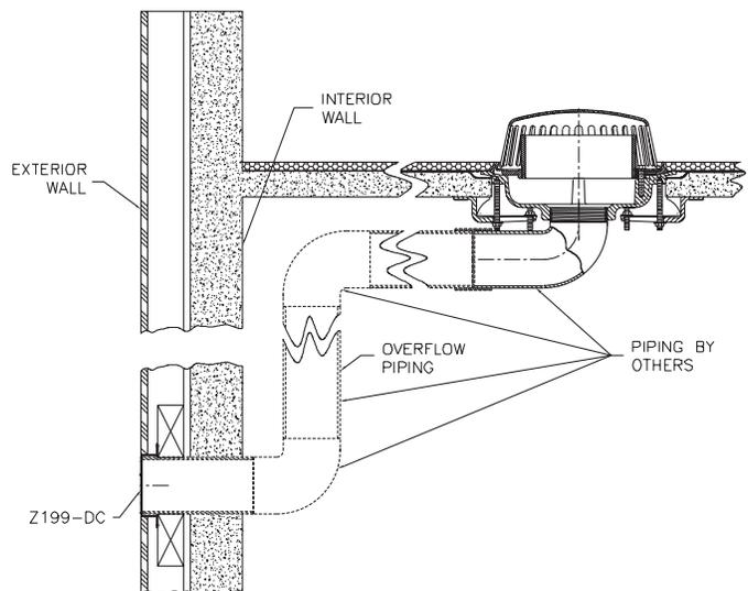
**Z101 HIGH CAPACITY 20" DIAMETER MAIN ROOF DRAIN**
