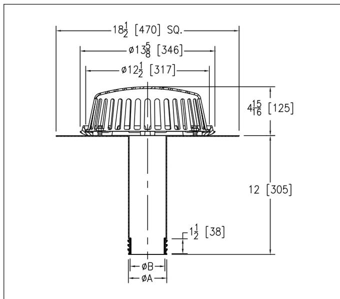
RD2150-FS Flat Sump Replacement Roof Drain
