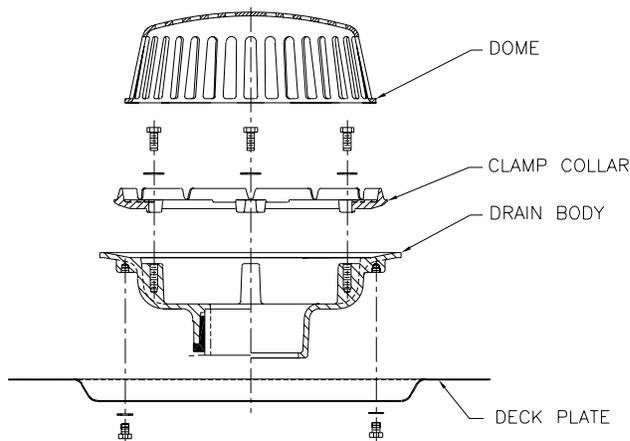
**Note:** Full installation is completed from the top of the roof deck, except for pipe connection.
