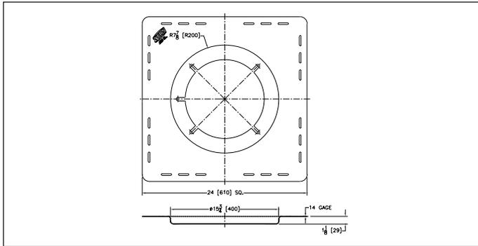
Unless the roof drain is poured directly into the concrete, the Underdeck Clamp (-C) is recommended to provide a secure, long lasting installation of the roof drain to your roof.
