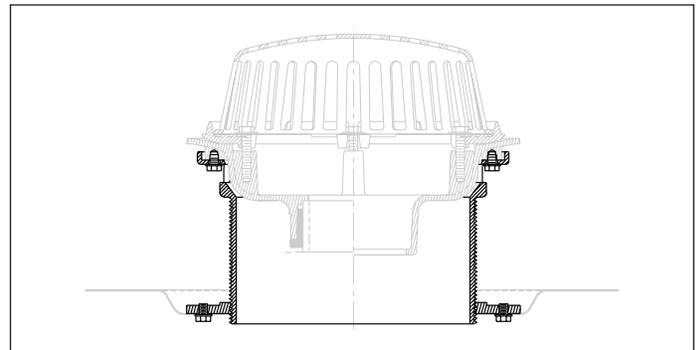
The -DR Top-Set Drain Riser Assembly is very similar to the -EA; however, the extension portion is completely removed from the path of the waterway.
