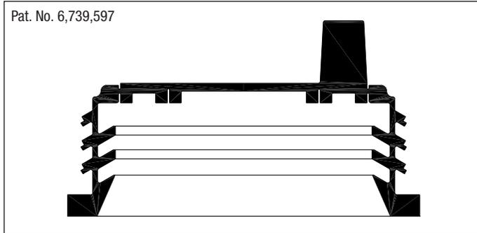
It is often required by plumbing codes that drain lines be tested for leakage once installation is complete. This test is typically performed by plugging all openings in the drain line system and applying a hydrostatic pressure charge of not less than 10-ft. head pressure to the lines for at least 15 minutes prior to inspection. The slightest loss of pressure in the system may indicate a possible leak.
