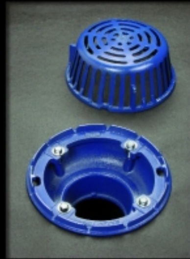
Seal Waterproof Membrane Under Clamping Collar. Simply Position Dome Onto Flashing Clamp.
