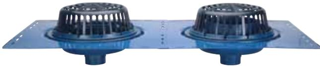
If code requires a primary drain and an overflow drain side by side, the Z163 (shown above) is an ideal solution. It can provide spacing to grid around the drains and easy installation with the Zurn Top-Set™ deck plate. The Z163 can also be incorporated with drain risers (-DR option) which allows for easy vertical adjustment.
