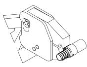
7) Check a completed connection with the appropriate sized section of the QickClamp Go gauge. Using the appropriate slot on the gauge for the fitting size, slide the gauge onto the crimped pinch ear. If the QickClamp pinch ear does not go into the Go gauge, the fitting should be cut out, the tool adjusted, and the fitting replaced.
