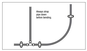
Zurn PEX straps and hangers hold pipe in position and prevent strain on fittings when the pipe is bent.
