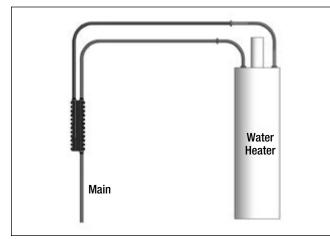
Supplying the water heater from the manifold.
