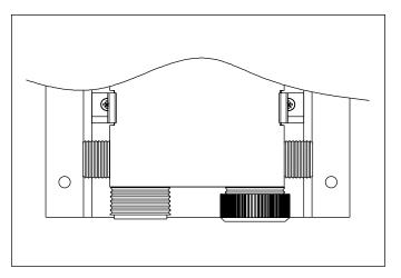
The 1" outlets can be fitted with a crimp x swivel or nut-ring-cone connector. These can then be used to supply high flow rate fixtures such as whirlpool baths, hose bibbs, etc. The unused 1" outlets need to be sealed using a 1" brass cap (Part No. QTC5FBG).
