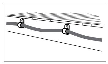
Always cut the pipe longer than necessary to allow some slack for any contraction in the pipe. 1/8'' per foot of length is usually enough.
