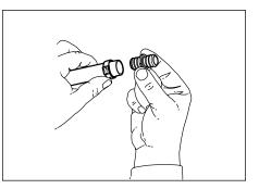
**3.** Push fitting into the tubing until the shoulder of the fitting is against the end of the tubing.
