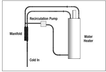
Recirculation pump with manifold.
