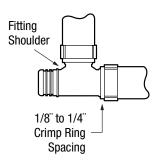
4. Position jaws squarely around the ring. Release upper handle to close jaws on the ring. Squeeze handles together to complete the crimp.
