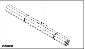
**Important: DO NOT** hook one tube to support the entire bundle. Straps should go around the entire bundle.
