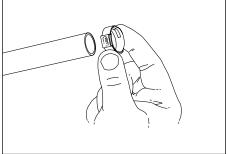
**2.** Slide the stainless steel clamp onto the tubing.
