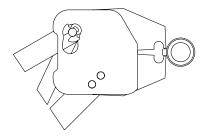
Open the QickClamp Medium Crimp Tool and remove it from the QickClamp. If the entire ear didn't crimp, **do not recrimp**. The crimp ring must be cut out and replaced.
