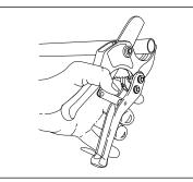
1. Measure and cut the tubing. Be sure you have a square, burr-free cut. An uneven or jagged cut may cause an improper connection.
