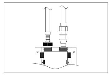
Connect the supply tubing to the appropriate header using one of the approved Zurn QickPort inlet/outlet connections as specified in the Zurn PEX product catalog.
