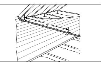
Straps can be as far as 6 feet apart if the pipe is continuously supported.
