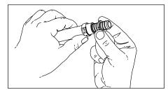
Position the stainless steel clamp so that it is 1/8" to 1/4" from the end of the tubing. Important: An improperly positioned ring may produce a weak condition.
