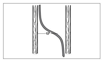
Since Zurn PEX tubing expands or contracts one inch for every 100 feet of pipe for every 10° of temperature change, you must allow for expansion and contraction in long runs with a 12-inch horizontal offset.
