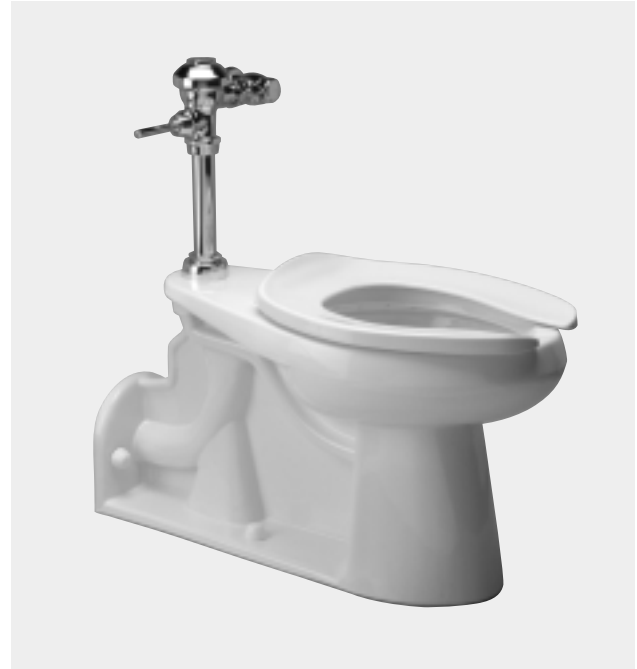
Z5640 1.6 gpf ADA height, elongated, floor mounted, back outlet flush valve water closet shown with Z5955SS-EL toilet seat and Z6000AV-WS1 flush valve (sold separately).
