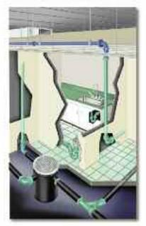
In 1999 Zurn introduced a complete line of polypropylene pipe and fittings for a variety of corrosive waste and chemical drainage applications. A major advantage of the Zurn system was the ability to use the same fittings for both mechanical and fusion installations.
