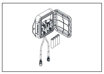
5. Connect the elecronic module to the connected monitior first, and the spout to the connected monitor second.
