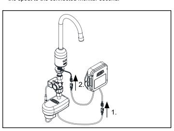
During initial installation, use the supplied lithium batteries. During subsequent battery changes, use either alkaline or lithium batteries; however, do not mix alkaline and lithium batteries together.
