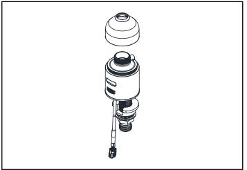
3. Align the small hole on the spout nut cover to the set screw to the back of the faucet body. Use the provided hex key wrench to lock the spout nut cover in place by turning in it clockwise.
