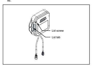
2. Loosen lid screw with supplied 3mm Allen wrench and Open the
