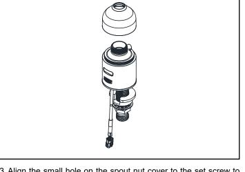
2.Install the spout onto the faucet body by turning the spout nut with an adjustable wrench clockwise. Feed the spout nut cover through the spout back onto the faucet body.
