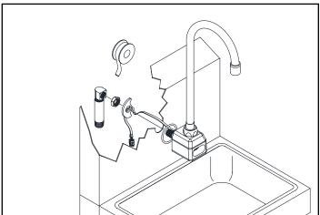
Note: Faucet location needs to be within 3 feet radius above electrical outlet for ACA configurations.
