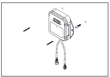
Install supplied lithium batteries. Close lid and secure by pressing on the lid tab until it snaps into place. Then tighten lid screw.
