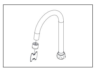
2.Install the spout onto the faucet body by turning the spout nut with a adjustable wrench clockwise.
