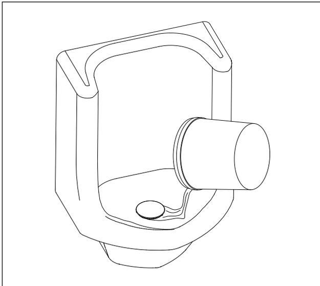
3.) Fill trapway with approximately 1 quart of water. Check drain line connections for leaks.
