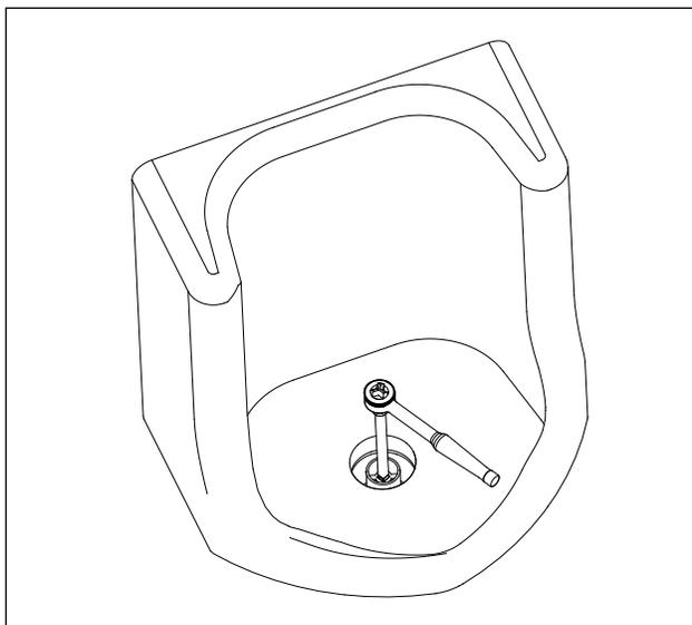
2.) Unscrew and remove bell trap. If the bell trap will not loosen by hand, use a 3/8" ratchet and extension, turning counterclockwise to remove.
