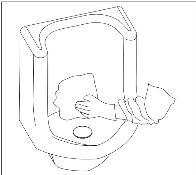
1.) Recommended daily maintenance of the Zurn Z5795/Z5796 urinal suggests wiping the walls of the urinal with a mild soap and water. Avoid dumping aggressive cleaners and/or large amounts of liquids down the urinal drain. Doing so may deplete the *AquaGreen™* sealant and allow sewer gases to back up into the restroom.
