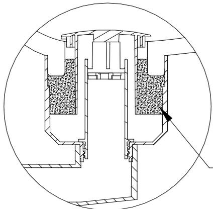
5.) **\*\* Important \*\*** Do not remove the strainer once Zurn AquaGreen™ sealant is in the trapway. Removal of the strainer will result in the loss of the sealant and reduce the life of the sealant.
