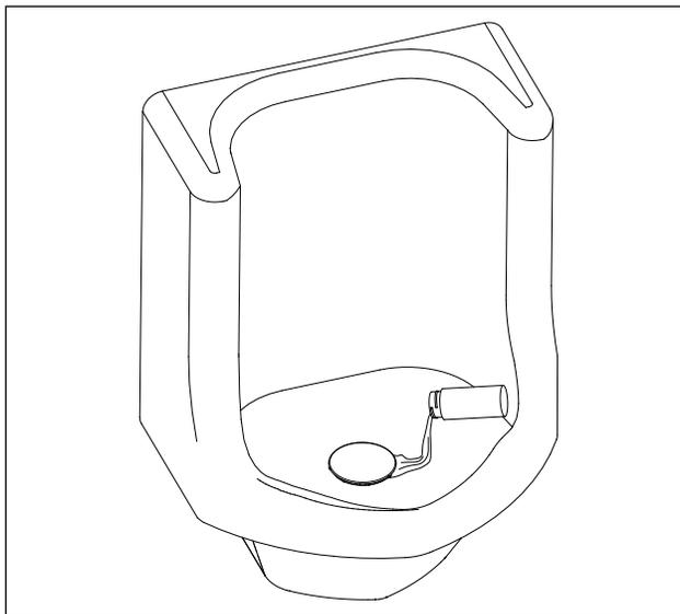
1.) It is critical that a layer of Zurn *AquaGreen™* urinal sealant be maintained at all times. To keep the Zurn Z5795/Z5796 urinal functioning properly and odor free, add 3 to 4 ounces of Zurn *AquaGreen™* sealant to the trap after every 3,000 uses.
