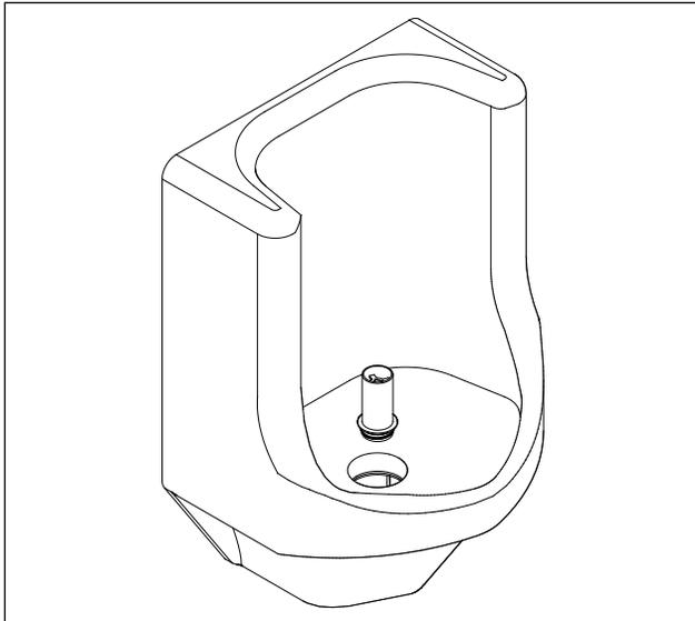
1.) Insert bell trap with o-ring (item 3) into urinal and turn clockwise to tighten. *Do not overtighten.*
