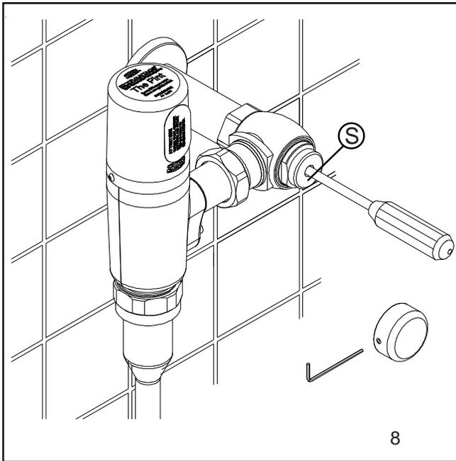
8.) The ZEG urinal valve comes preset for both flow volume and sensing distance. Each valve is operated at the factory using water to insure proper function before being packed for shipment. The valve does not require water pressure regulation for variation in water pressure within the specified pressure range (20 psi to 120 psi) due to internal pressure regulation.
