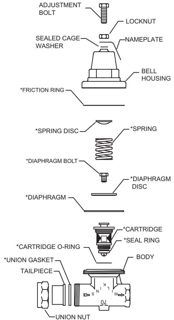
**Regulators in series:** Where the desired pressure reduction is more than a 4 to 1 ratio (i.e. 200psi to 50psi), multiple regulators in series should be installed.
