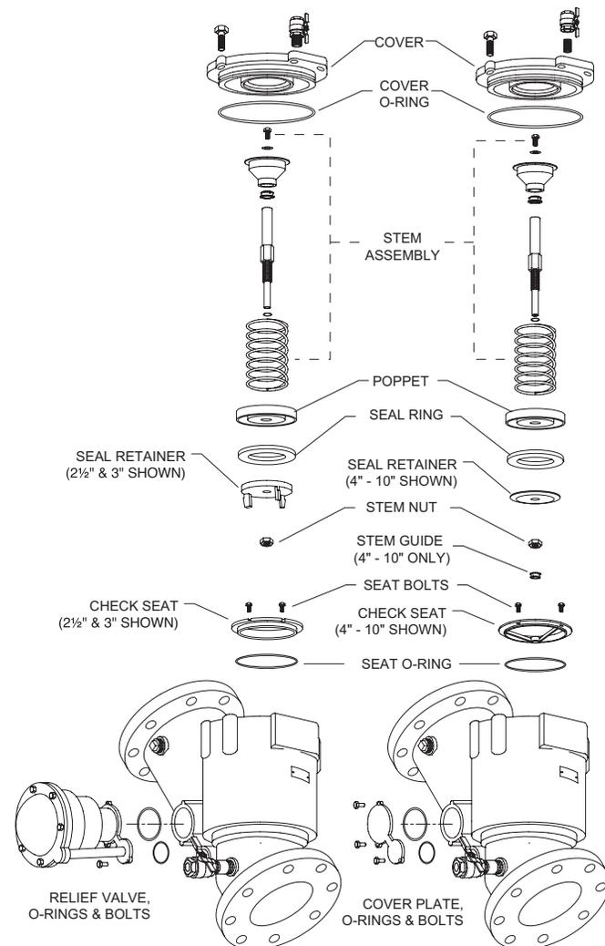
wrench. NOTE: Poppets are self contained. The covers should lift no more than 1/2" before tension is relieved.
