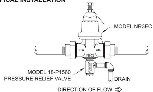
**Regulators in series:** Where the desired pressure reduction is more than a 4 to 1 ratio (i.e. 200psi to 50psi), multiple regulators in series should be installed.
