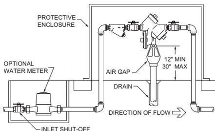
**CAUTION:** Do not pipe the relief valve solidly to a floor drain, sewer or sump.
