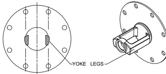
**NOTE:** Line up diaphragm screw holes with holes in body. Move yoke up and down checking for yoke contacting or dragging on valve body.
