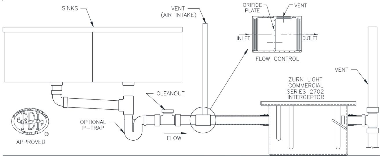
Zurn Light Commercial Series Grease Interceptors GT2702 consist of a interceptor rated at ( ) gpm and a properly sized flow control fitting.
