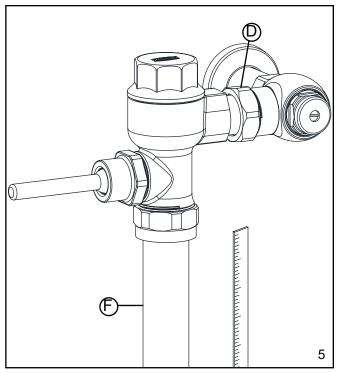
5.) Determine the length of the vacuum breaker tube (F) required to join the flush valve and fixture spud. Cut the vacuum breaker tube, if required, to this length. Assemble the vacuum breaker tube assembly and spud nut assembly to the flush valve and fixture spud.
