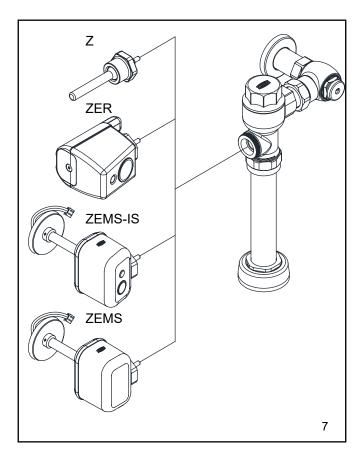
7.) Attach the appropriate handle/actuator to the valve body.
