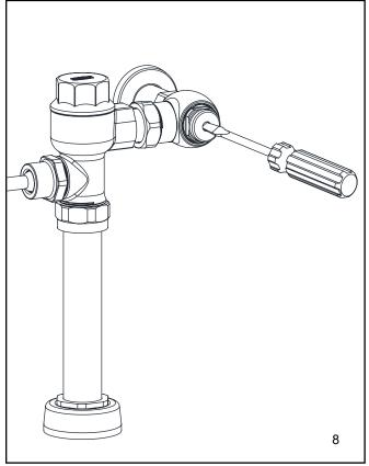
**8.)** Determine all flush valve connections are tight and proceed to open control stop.
