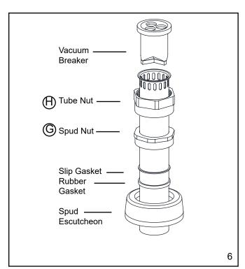
6.) Hand tighten spud nut (G) to the fixture and vacuum breaker tube nut (H) to flush valve. Adjust the valve assembly for plumb. Tighten fixture spud nut (G), vacuum breaker tube nut (H) and lock nut (D) (fig. 5) with a wrench.
