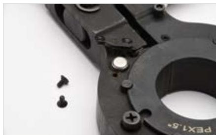
2. Gently move the battery cover to the side, exposing the two batteries, which are stacked one on top of the other. Be careful not to damage the wire that's attached to the battery cover.
