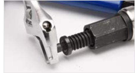
1. If necessary, remove existing reverse thread screw (#6), from the tool, by placing a wrench on the flat sides of the screw head. Turn the screw clockwise until the reverse thread screw and the guide/stop washer, are no longer attached to the tool.
