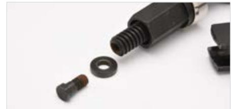
2. To install the new reverse thread screw (#6) and guide/stop washer (#7), you must first place the guide/stop washer onto the reverse thread screw. Thread the screw with washer into the tool by turning the screw counter clockwise with your fingers. Place a wrench on the flat sides of the reverse thread screw head and turn it counter clockwise until tightened completely. Run the screw/nut up and down the threaded shaft several times by hand, to verify proper operation.
