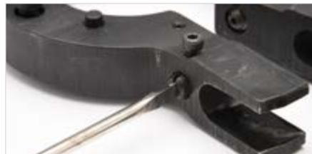
2. To install the new jaw stop screw (#5) into the tool, you must first engage the jaws, as you would when making a crimp, until the LED light comes on. Using a slotted screw driver, thread the jaw stop screw into the tool, clockwise, until the screw stops when it touches the other side of the tool. Turn the
