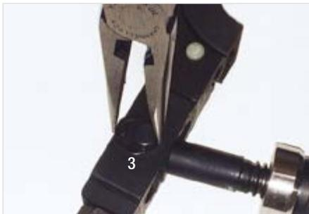
2. To install a new E-Clip (#3), place the E-Clip (#3) on the surface of the tool with its opening positioned around the groove of the pin. Use needle nose pliers to push the E-Clip (#3) onto the pin until it snaps into place. (Note: The E-Clip will rotate freely but should not come off without prying with force.) Follow same procedure for E-Clip #2 (see above diagram for E-Clip #2 location).
