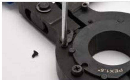
1. To replace the batteries, (that power the LED light), use a Phillips head screwdriver to remove the two screws that hold down the cover by rotating them counter clockwise.
