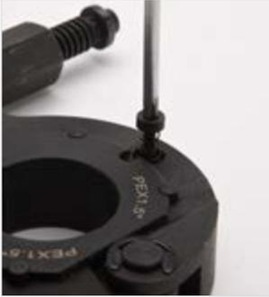
1. If necessary, remove existing spring/pin jaw retainer (#4), from the tool, by using a Phillips head screw driver to rotate the screw counter clockwise. (Note: The spring around the pin is also removed.) Lift the tool from the work surface to reveal the jaw retainer, that was attached to the pin, laying on the work surface. You can now remove the jaw from the tool.
