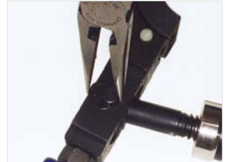
(We recommend an extreme pressure lubricant such as white Lubriplate or the lubricant sold for the screw drives of Genie garage door openers.) To apply lubricant, turn the nut counter clockwise by hand until it stops at the end of the screw. Apply a small amount of lubricant to the threads at the midway point of the screw. Spin the nut up and down the screw a few times by hand to distribute the lubricant. Wipe off any excess lubricant with a rag.
