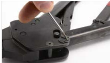
2. Remove existing E-Clip (#4) by prying it away from the pin with a flat head screw driver or needle nose pliers.
