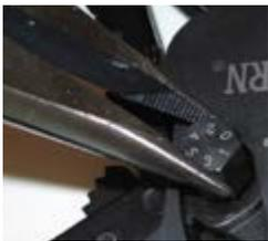
off without prying with force.) Apply a lubricant to the moving parts. Perform a crimp and check with gage. If crimp does not gage properly, remove E-Clip, push pin far enough so it can be turned, then position the pin so that the next sequential number on the pin is facing the dot on the tool. Push the pin while jiggling the handle to seat the pin. Install E-Clip (#4). Repeat until crimp gages properly.
