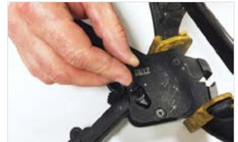
1. Clean the adjustment pin area of the tool with a brush and rag to remove any dirt and surface rust. Be careful not to remove the adjustment dot marking on the tool.
