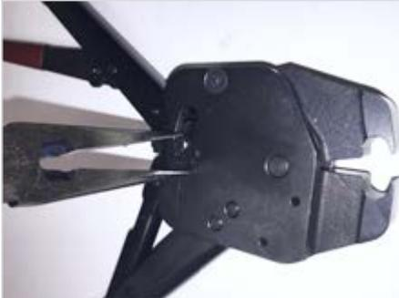
3. Remove the ratchet bar clamp to release the jaws. Turn the tool over to expose the other side of the pin. The groove in the pin should be above the surface of the tool. Place the E-Clip (#4) on the surface of the tool with its opening positioned around the groove in the pin. Use needle nose pliers to push the E-Clip onto the pin until it snaps into place. (Note: The E-Clip will rotate freely but should not come
