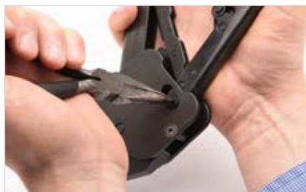
3. Tap the adjustment pin (#3) out as far as you can with needle nose pliers then remove pin by hand using a pulling/wiggling motion.
