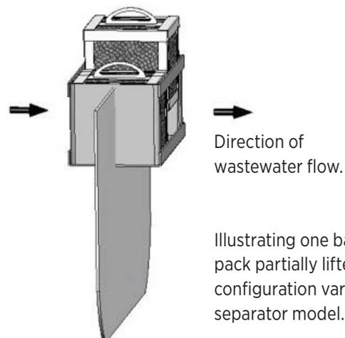
Illustrating one baffle pack partially lifted. Pack configuration varies with separator model.
