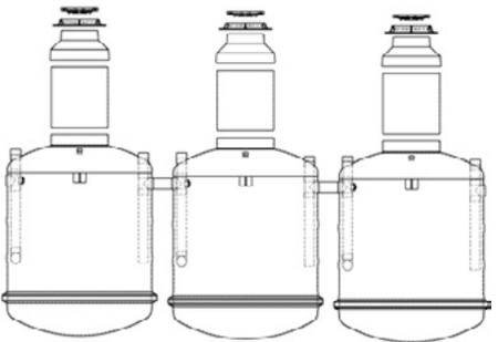
Figure 2.2: Triple tank with one accessway per tank
