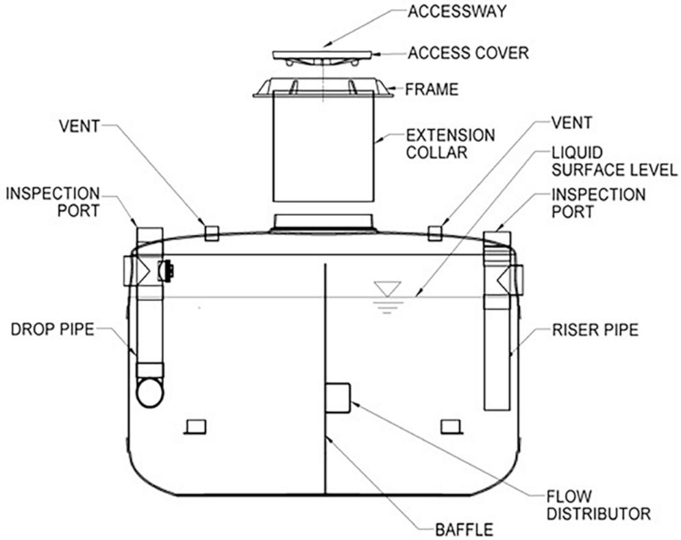
Figure 1: Single tank Proceptor design
