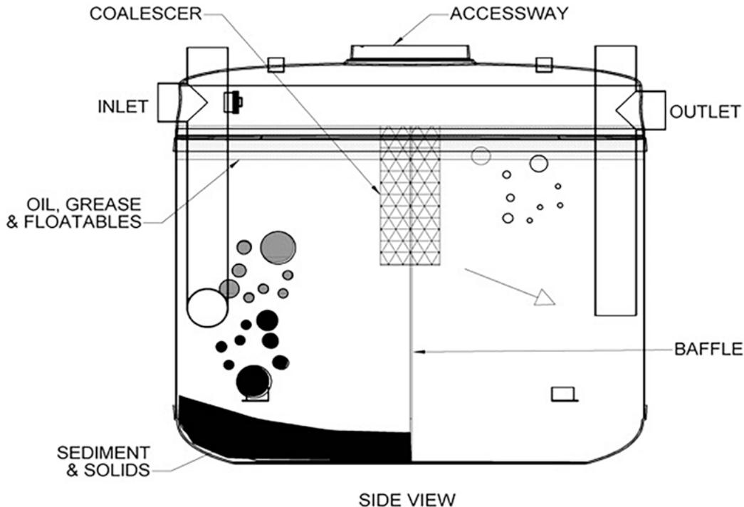
Figure 5: Proceptor separator with coalescer
