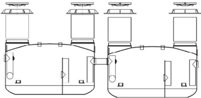
Figure 2.4: Dual tank with dual accessway
