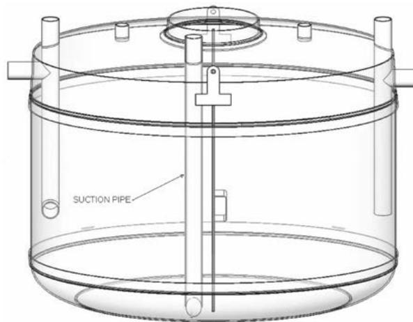
**Figure 7: Proceptor with suction pipe option**
