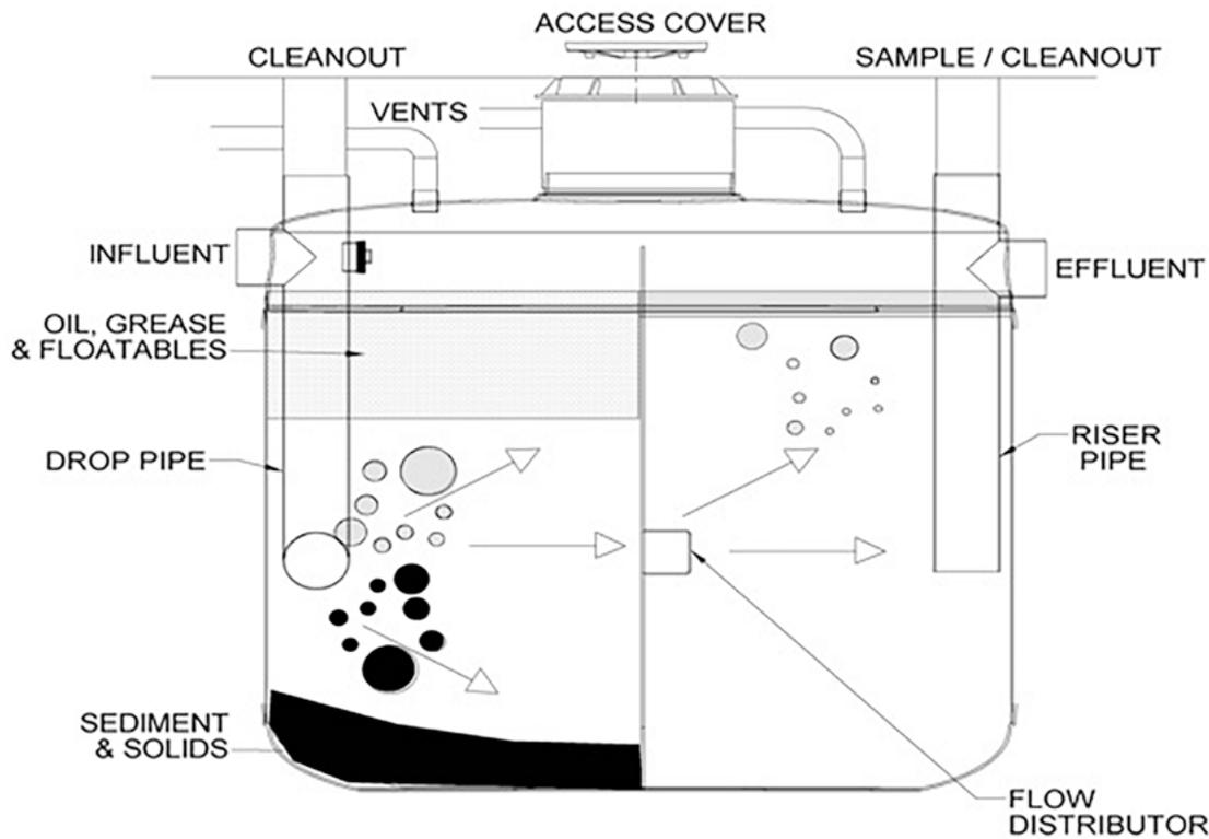
Figure 3: Proceptor operation: process flow dynamic
