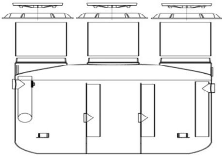
Figure 2.5: Single tank with triple accessway
