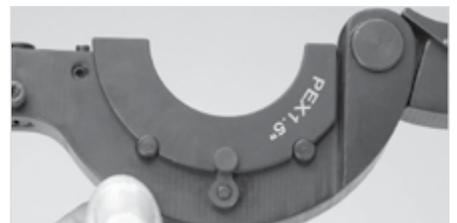
4. Push spring/pin while rotating jaw retainer clockwise until jaw retainer lines up with notch in jaw. Release spring/pin to lower the jaw retainer into the notch to lock the jaw in place. Repeat for other jaw.
