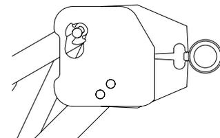
**Crimp jaw must completely cover the length of the crimp ear before crimping.**
