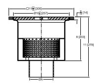
Three anchor tabs spaced 120 degrees apart not represented in cross section view.
