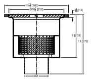
Three anchor tabs spaced 120 degrees apart not represented in cross section view.
