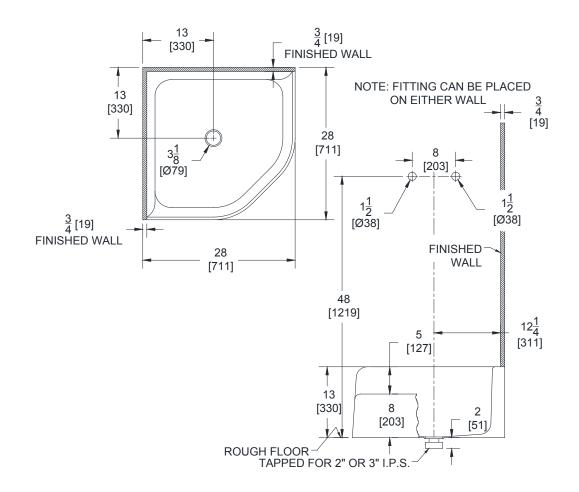
Fixture dimensions meet ASME A112.19.1 / CSA B45.2 requirements.
