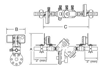
\* Note: The BVMS 3/4" - 1" Configuration requires a minimum of 2" straight pipe on either end to allow the switch to be mounted above the ball valve "T" handles.
