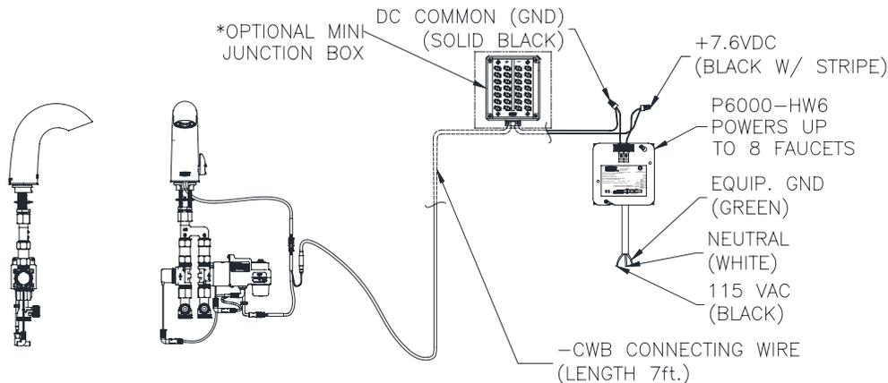
OPTIONAL: \* P6000-MJ mini junction box streamlines wiring for connecting up to 8 faucets to the P6000-HW6 power converter.
