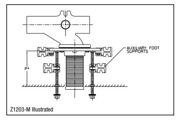
**-PA** Adjustable Coupling Connection for Penal Fixtures (Z1214 and Z1215)
