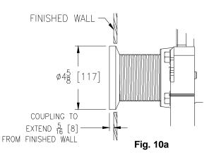
b. <u>EZ-Set<sup>™</sup> Coupling</u> - Thread the coupling into the faceplate by hand until it engages the o-ring and begins to resist. Using a strap or pipe wrench, continue to turn the coupling into the o-ring to create a water-tight seal. Ensure the protective sleeve is flush with the test cap. See Fig. 10 & 10b
